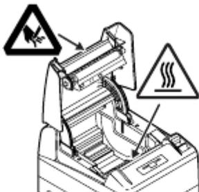
THESE LABELS INDICATE THE RISK OF ANY INJURY DUE TO "HIGH TEMPERATURE" OF THE PRINT HEAD AND "SAW-TOOTHED EDGE" OF THE MANUAL CUTTER.
